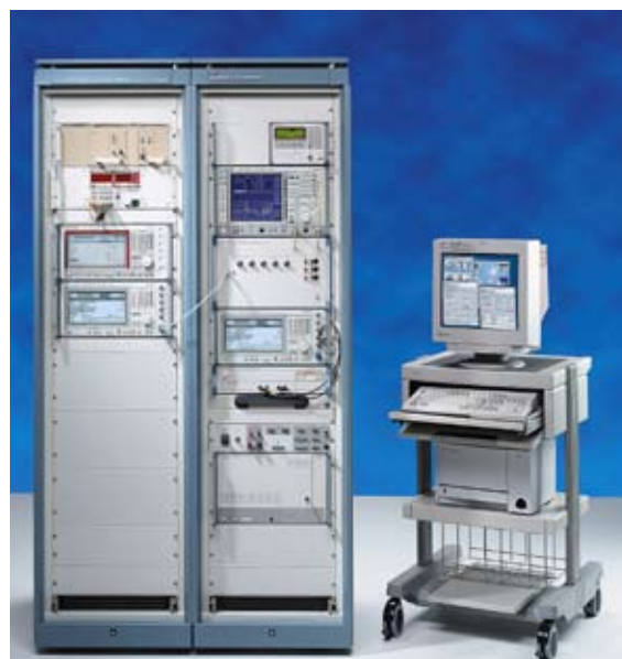
2G/3G conformance testing with the R&S®TS895xGW family
